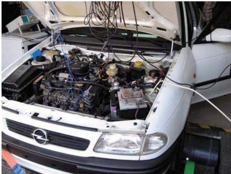
Fig. 2. Engine compartment of tested vehicle
